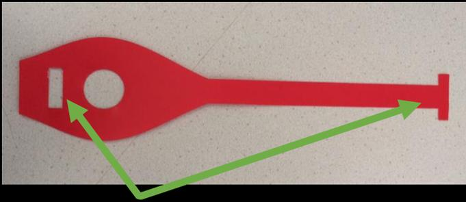
When the 'T' shaped end looped through the rectangular hole, it would slip out very easily.
